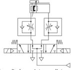
System to stop the cylinder on intermediate position with higher tolerances.
